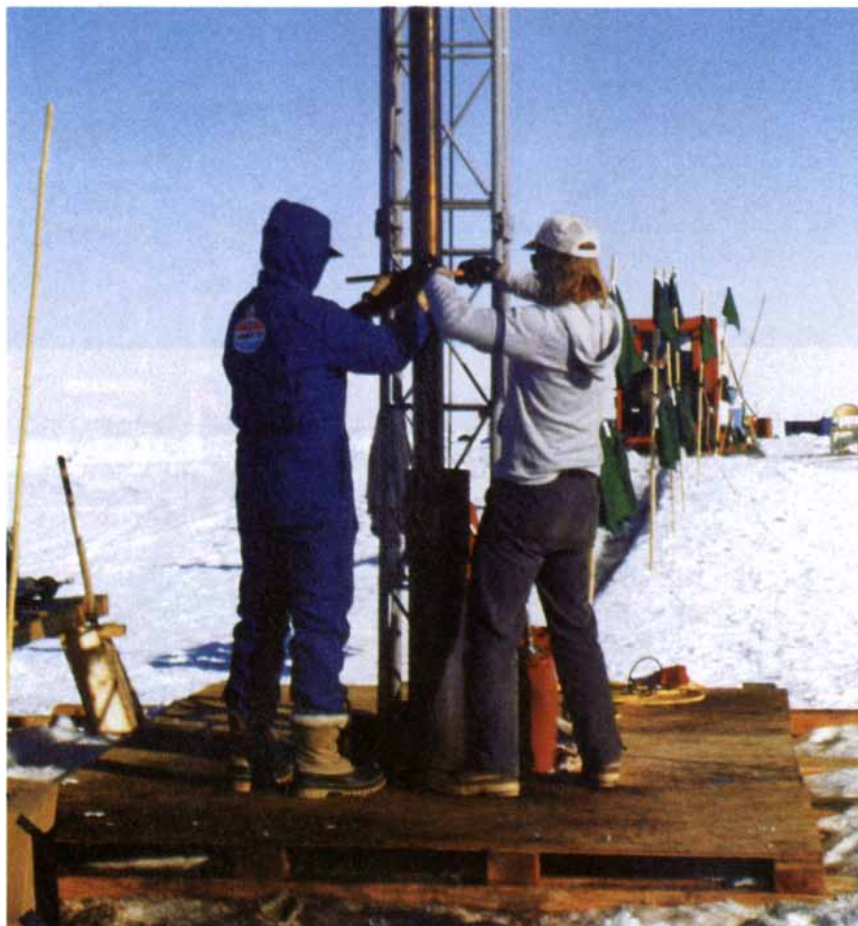
GRAVITY METER is carefully hoisted out of a deep borehole in the Greenland ice sheet a few miles south of the Arctic Circle. The half-million-dollar device measures local gravitational force at various positions to a depth of 1,600 meters with a precision of one part in 100 million. The meter, which is normally used for petroleum prospecting, is testing for the possible existence of new gravity-related interactions. Seen in the photograph are Casey Rohn of the University of Nebraska's Polar Ice Coring Office and James Wirtz of Amoco. Ted Lautzenhiser is inside the red winch-operating cabin.
