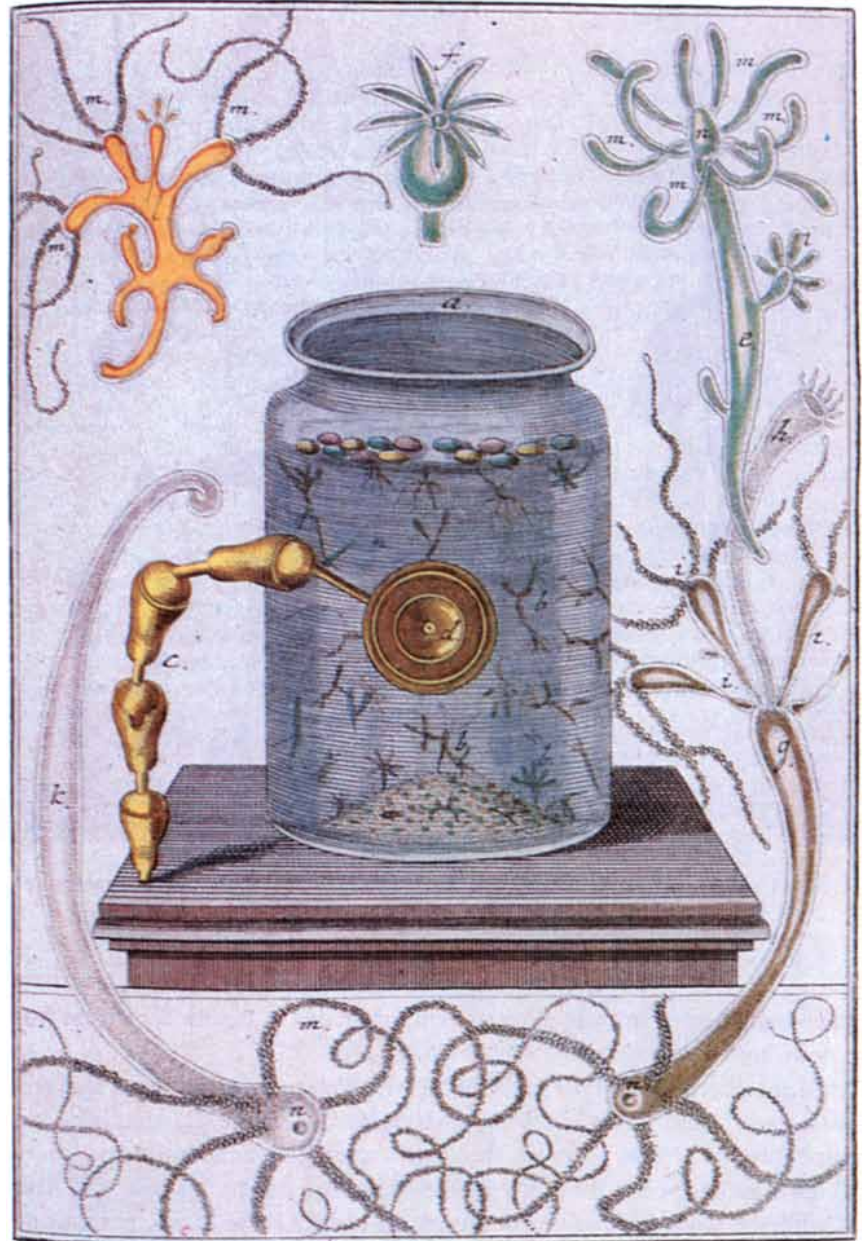
TREMBLEY'S MICROSCOPE was no more than a single lens mounted on a multijointed arm. The drawing, made by Martin F. Ledermüller in about 1762, also shows Trembley's favorite receptacle for his hydras surrounded by (clockwise from top left) a hydra monster, a contracted and a relaxed green hydra and specimens that may be Hydra oligactis .
