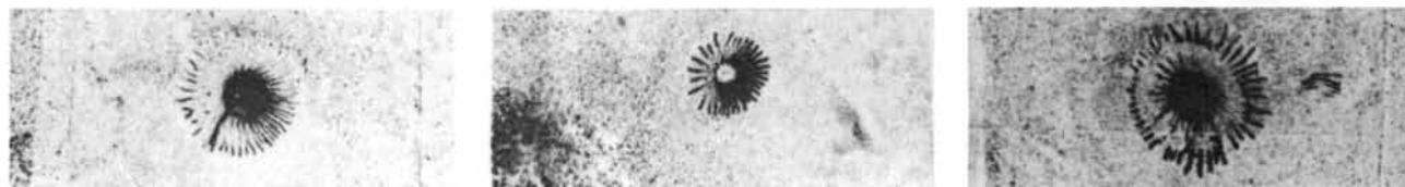
Lichtenberg figures made by a hand-held pinhead (left), pinpoint (middle) and scissors point (right)
