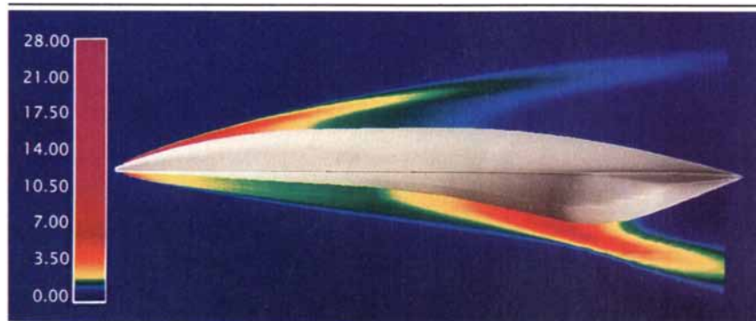
COMPUTER SIMULATION of airflow around a proposed X-30 aircraft flying at Mach 12.4 shows the formation of compression zones. Highest pressures are magenta, lowest are blue. The work was done at NASA's Ames Research Center.
