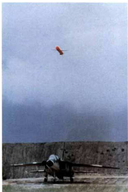
TOMAHAWK CRUISE MISSILE launched from a submerged U.S. submarine more than 400 miles away explodes above an aircraft on San Clemente Island, Calif.
