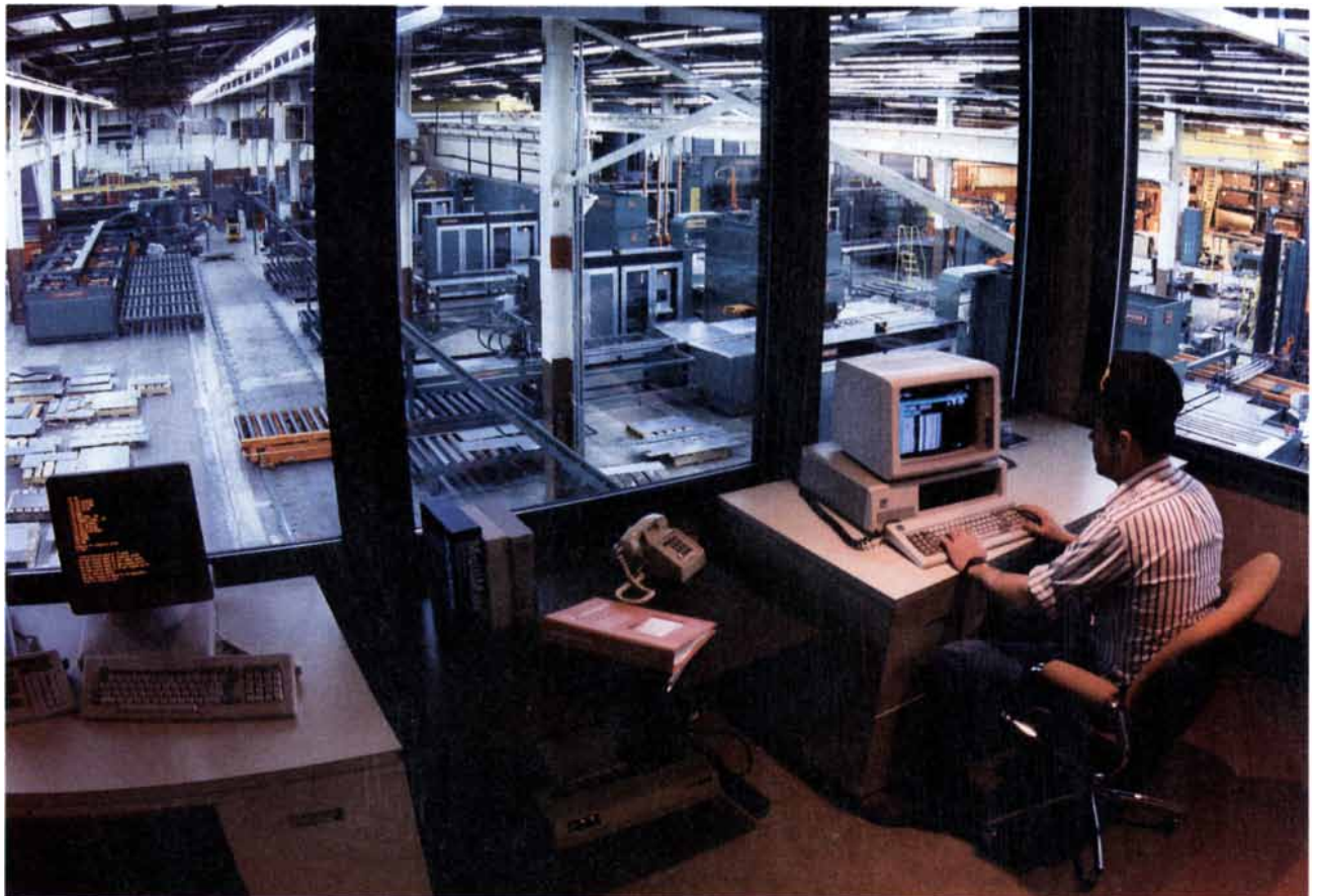
FLEXIBLE MANUFACTURING approach applied in the production of lighting panelboards at the Salisbury, N.C., plant of
