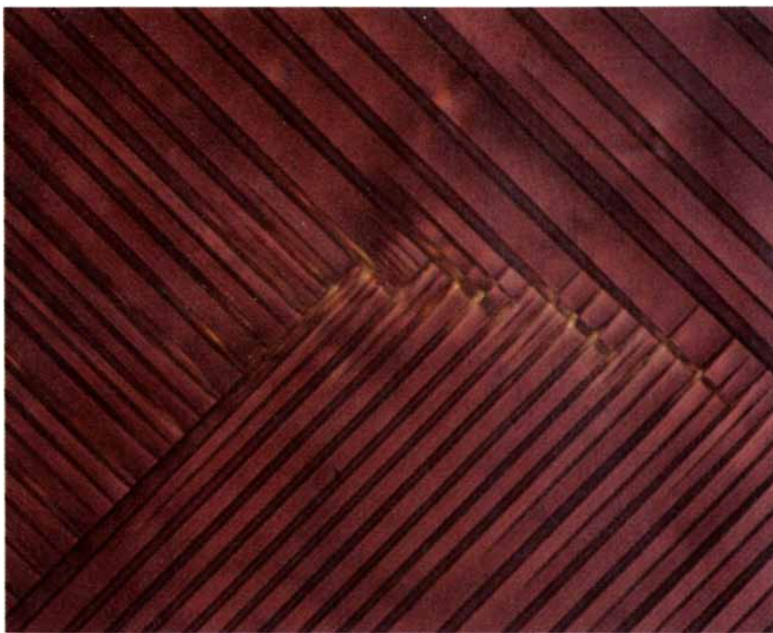
CROSS SECTION of a barium titanate crystal reveals a common defect in perovskites: twinning, or the formation of essentially identical domains that are oriented differently. Here the differing stripe patterns in the two large domains reflect differences in the titanium off-centering that is characteristic of barium titanate. The titanium atoms in adjacent light and dark bands are shifted in opposite directions. The sample, which was provided by Robert D. Shannon of E. I. du Pont de Nemours & Company, Inc., appears purple because it was photographed under polarized light.
