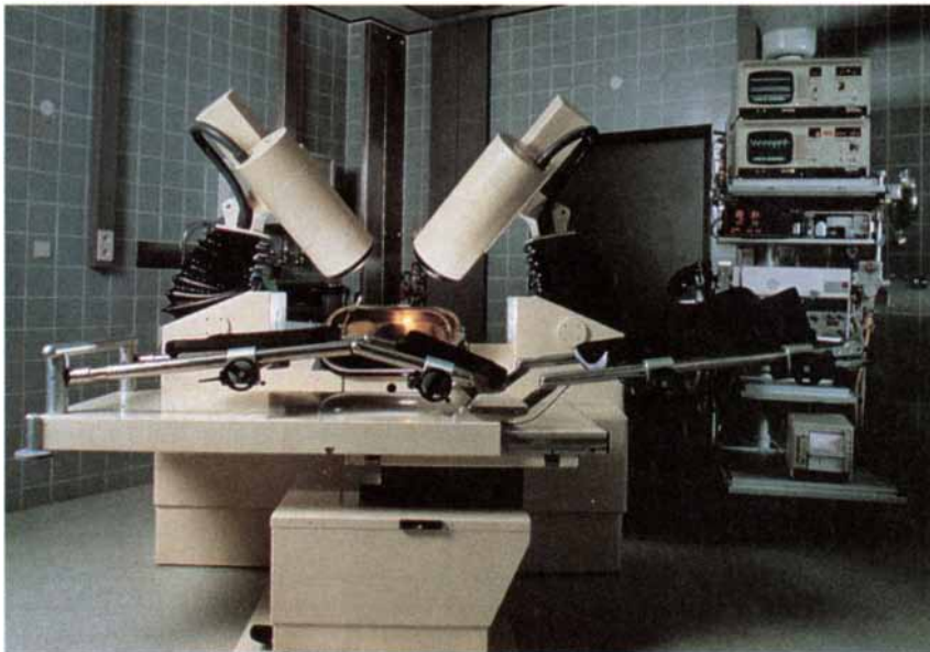
The lithotripter, built by West Germany's Dornier company, crushes kidney stones by aiming sonic waves at them. The first lithotripter was approved by the Food and Drug Administration for U.S. distribution in 1986.
