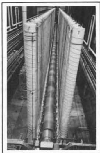
A gas centrifuge cascade
