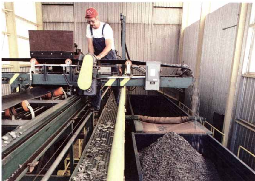
RECYCLING of paper can significantly reduce the amount of waste. This recycling plant shreds paper that is later converted into paper towels, newsprint and flowerpots.
