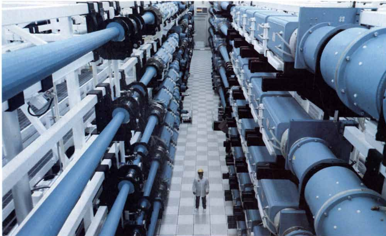
NOVA LASER at the Lawrence Livermore National Laboratory is the world's most powerful optical laser. It can deliver 100,000 joules of energy in less than one-billionth of a second, a 10^{14} -
