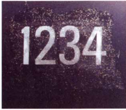
TAGGING SYSTEM for missiles was developed at the Sandia National Laboratories. An identification number on a missile's casing is covered with a hard epoxy resin containing random, reflective particles of mica. The reflections under light from different angles (compare the left and right images) form a unique signature.
