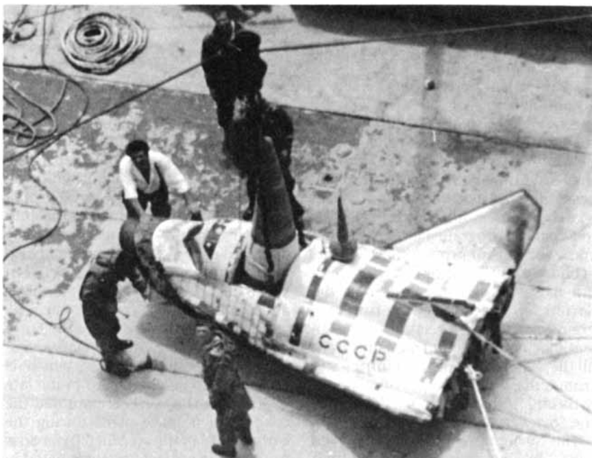
SUBSCALE SPACE PLANE was photographed from a Royal Australian Air Force plane flying over a Soviet ship in the Indian Ocean. The people on the ship's deck are retrieving the model from the water, where it had landed after a test flight. The actual size of the space plane is probably about two or three times the size of this model.
