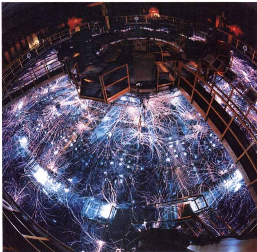
ELECTRICAL DISCHARGES lace the surface of water bathing the Sandia National Laboratories' Particle Beam Fusion Accelerator II as it fires a pulse of light ions. The Department of Energy is considering employing such a machine as a "driver" for an advanced inertial-confinement facility. Its million-joule beams are more powerful than any laser's, but they are also much more difficult to focus.
