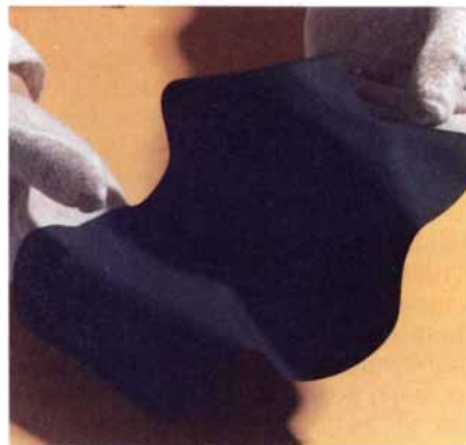
SUPERCONDUCTING TAPE AND WIRE have been fabricated by Roger B. Poeppel and his colleagues at the Argonne National Laboratory. Before sintering, the tape (left) is soft enough to be molded into various shapes; after sintering it becomes extremely brittle. A modest amount of flexibility has been achieved in a sintered coil (right).
