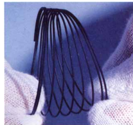
SUPERCONDUCTING TAPE AND WIRE have been fabricated by Roger B. Poeppel and his colleagues at the Argonne National Laboratory. Before sintering, the tape (left) is soft enough to be molded into various shapes; after sintering it becomes extremely brittle. A modest amount of flexibility has been achieved in a sintered coil (right).
