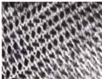
POROUS STRUCTURE of macromolecular crystals is evident in an electron micrograph of a crystal of a bacterial enzyme (above). The dark channels are clearer in the enlargement (left). The channels make the crystals extremely fragile, but they also provide paths for the diffusion of small molecules. In the photograph below, color is supplied not by polarized light but by a red drug that has penetrated the solvent channels in the crystal and has bound to the molecules forming the lattice.
