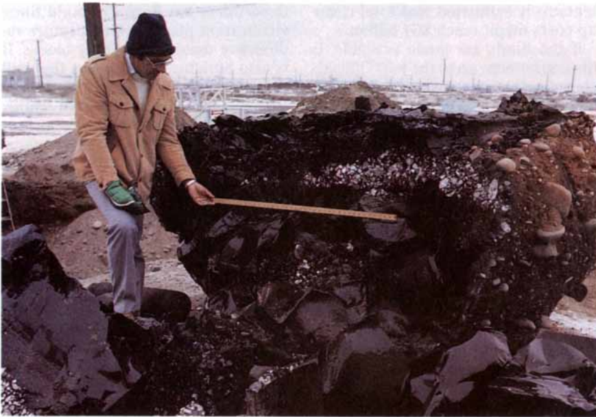
VITRIFICATION PROCESS being developed by workers at the Battelle Pacific Northwest Laboratories converts soil into an obsidianlike substance.
