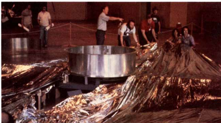
PROTOTYPE SOLAR SAIL , made of Mylar, might someday soar in space powered only by photons. The circular bus at the center would carry instruments. Photograph courtesy of Robert L. Staehle of the World Space Foundation.
