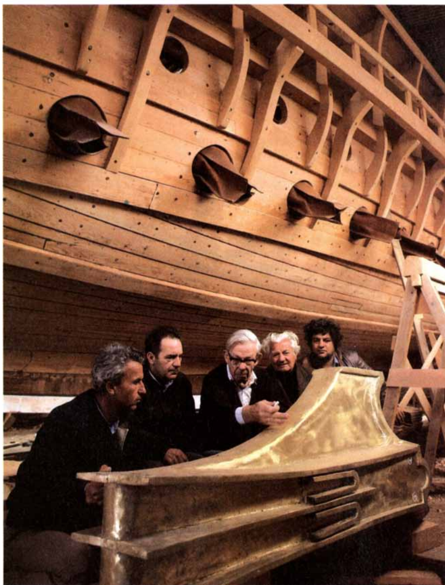
HULL VIEW of Olympias shows the smooth construction and shallow draft of the ship. Leather sleeves cover the lowest oar ports, which are only .4 meter above the waterline. A projecting outrigger provides the pivots for the topmost file of rowers. In the foreground the author ( middle ) discusses the shape of the ram with colleagues.
