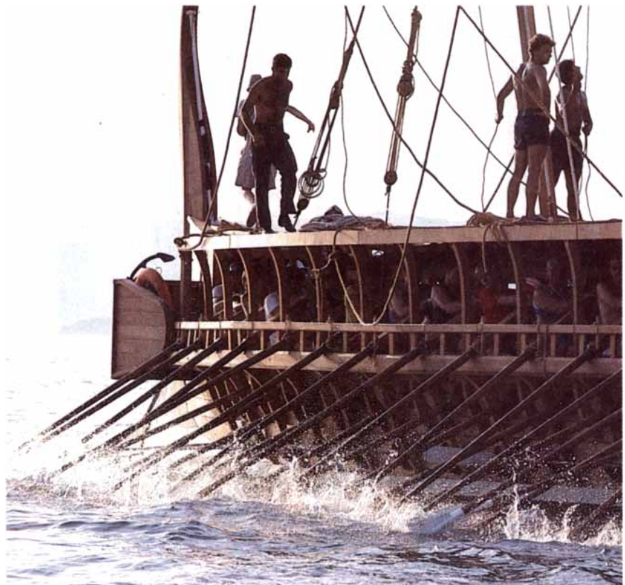
ALL THREE TIERS of rowers attack the water with their oars as they drive Olympias into a sprint. In sea trials the ship proved itself capable of more than nine knots under oar or sail. Coaches, recorders and assistants stand on the canopy deck.
