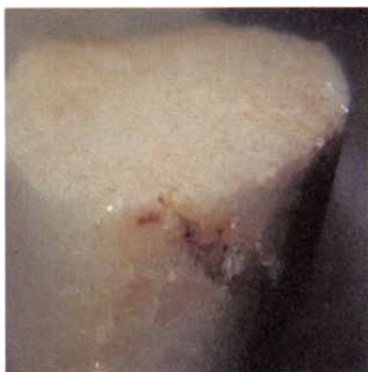
CORE SAMPLE the size of a pencil eraser ( left ) was drilled from a weathered fracture at the right knee of the kouros. Reddish iron oxide stains the calcite crust on the exposed surface and penetrates deeply into a fissure; the fresh dolomite is snow-white. A scanning electron micrograph ( right ) shows the tight bonding of the calcite crust to the underlying columns of dolomite crystals, here enlarged 1,500 diameters.
