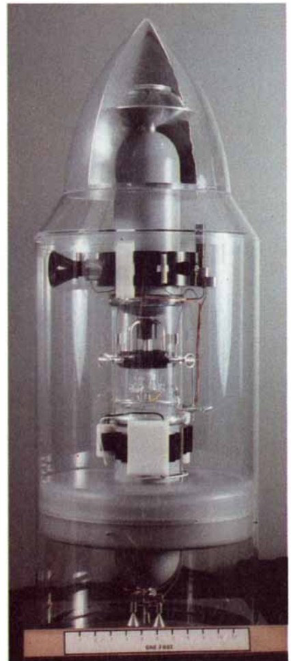
BRILLIANT PEBBLE , a space-based rocket designed for antimissile defense, could also destroy satellites.
