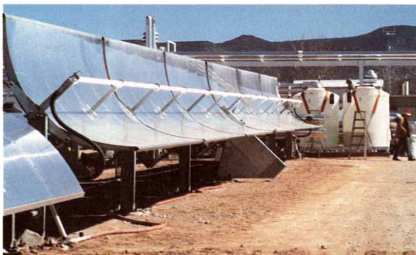
TROUGH-SHAPED MIRRORS focus sunlight on tubes containing contaminated water. The ultraviolet energy in sunlight initiates a reaction that destroys organic contaminants in the water. Photograph courtesy of Sandia National Laboratories.
