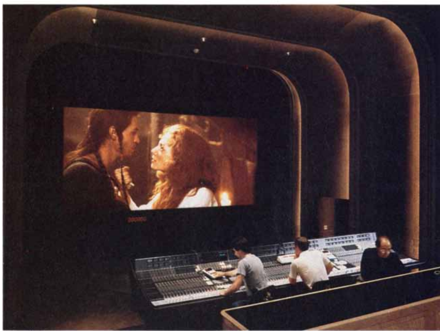
MIXING STUDIO at Sprocket Systems in San Rafael, Calif., allows workers to synchronize sound and picture and to manipulate sound recorded on as many as 40 separate magnetic tracks. Much of the work currently done on the mixing boards could be superseded by sound editors employing digital technology.
