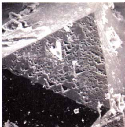
KOUROS DOLOMITE'S distinctive crystal structure, shown in a polarized-light micrograph ( left ), is consistent with dolomite from Thasos. A scanning electron micrograph of a core sample ( right ) shows triangular pits etched by corrosive groundwater over a long time on the face of a dolomite crystal (enlarged 300 diameters).
