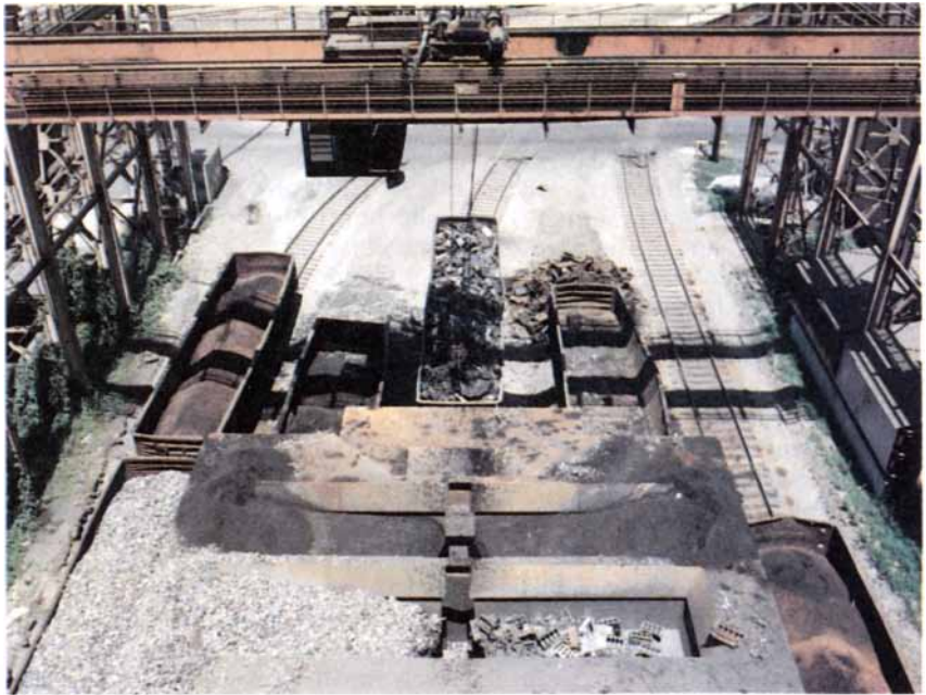
SCRAP METAL from the casting and machining of engine parts awaits recycling at a General Motors foundry in Defiance, Ohio. The company operates four foundries; they are supplied entirely by scrap from sheet-metal stamping, iron casting and machining operations. Despite the relative ease with which scrap can be recycled, millions of tons pile up every year in U.S. scrapyards for lack of ready markets.
