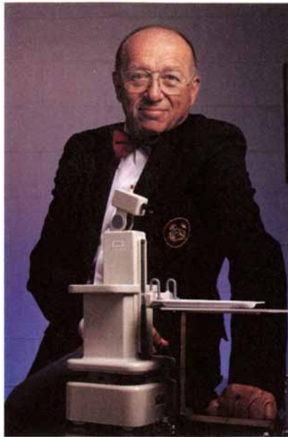
ROBOT POSES WITH ITS CREATOR, Joseph F. Engelberger. The robot—an early model—was designed to deliver dinner trays directly to hospital patients. Engelberger is working on larger robots that will wash and vacuum floors. Photograph by Wayne Sorce.
