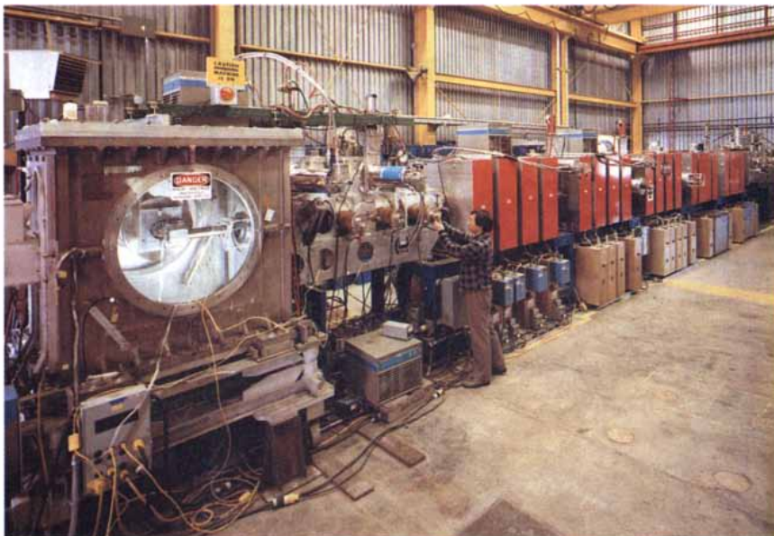
MULTIPLE-BEAM EXPERIMENT (MBE-4) is a heavy-ion accelerator at the Lawrence Berkeley Laboratory. Whereas most accelerators boost particles by means of powerful radio waves, the MBE-4 employs induction. Ions are generated in the box with the window at the left and accelerated in the red boxes at the right.
