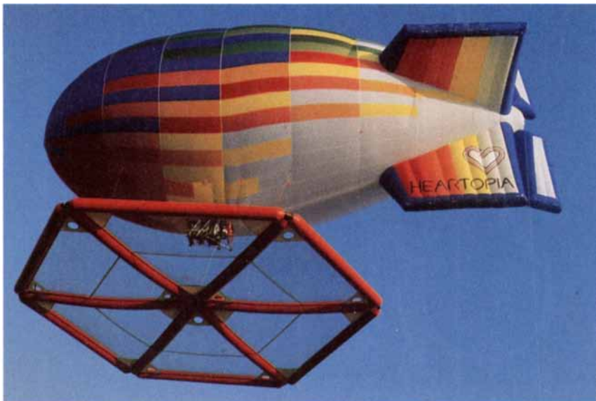
RAFT for studying the rain-forest canopy is carried aloft by a hot-air balloon. The equipment was designed by Francis Hallé of the University of Montpellier II.
