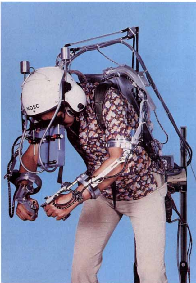
"GREEN MAN" teleoperator enables a human being (left) to operate a humanlike workstation (right) from a distance. Two television cameras on the station send information to two miniature helmet-mounted television screens positioned directly in front of the operator's eyes; sound is transmitted as
