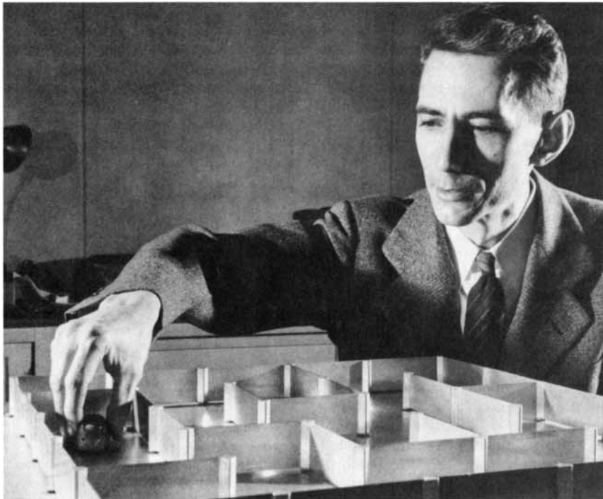
THESEUS , a mechanical mouse, is shown with its inventor, Claude E. Shannon, in a 1952 photograph from Bell Laboratories. The mouse "learns" to find its way out of a maze with the help of a magnet guided by circuitry beneath the maze.
