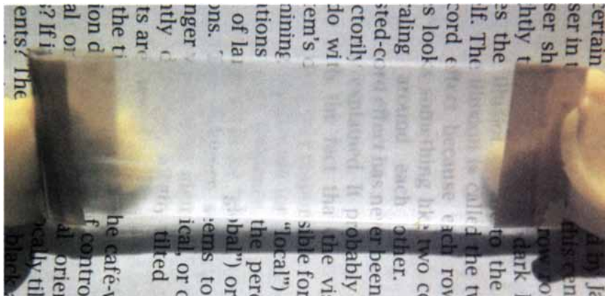
The necked region of a polymer sheet obscures print
