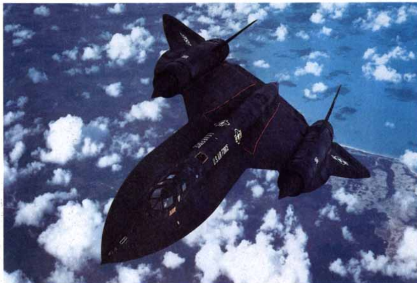
SR-71 BLACKBIRD measures 107 feet from tip to stern and 56 feet across the wings.
