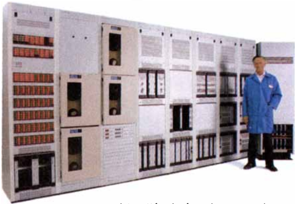
Motorola's EMX family of switches are now the most widely used cellular telephone switching systems in the world.
