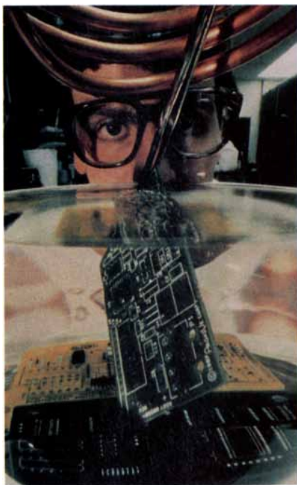
ALTERNATIVE CLEANING AGENTS for printed-circuit boards, intended to replace chlorofluorocarbons, are being developed at a Du Pont laboratory near Wilmington, Del.
