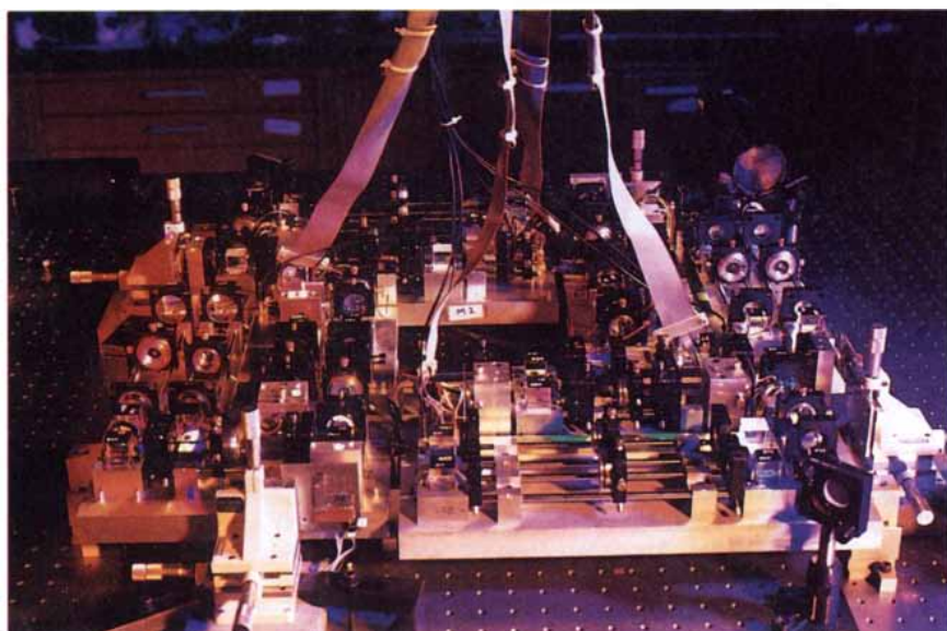
EXPERIMENTAL DIGITAL OPTICAL PROCESSOR —which has about as much data-processing capacity as a semiconductor chip controlling a dishwasher—uses beams of infrared light generated by laser diodes instead of electrons to process data. Photograph courtesy of AT&T Bell Laboratories.
