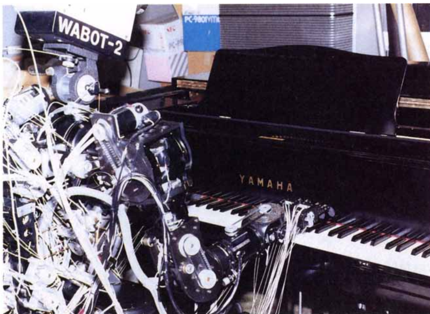
TEN-FINGERED WABOT , a robot built by engineers at Japan's Waseda University, can tap out a tune on the piano after scanning the sheet music for 15 seconds. It also takes requests. Photograph by Frederick S. Myers.
