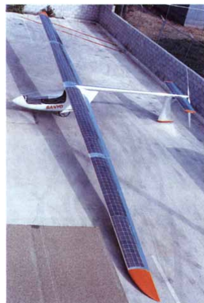
SOLAR AIRPLANE is powered by sheets of flexible, lightweight solar cells.
