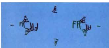
Two lens systems graphically reverse the quadratic transformation that defines the Julia set. The lenses perform the transformations +(z - c)^{1/2} and -(z - c)^{1/2} , the inverses of z^2 + c . The limiting image of the copying machine is a Julia set.
