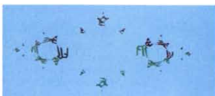
Two lens systems graphically reverse the quadratic transformation that defines the Julia set. The lenses perform the transformations +(z - c)^{1/2} and -(z - c)^{1/2} , the inverses of z^2 + c . The limiting image of the copying machine is a Julia set.
