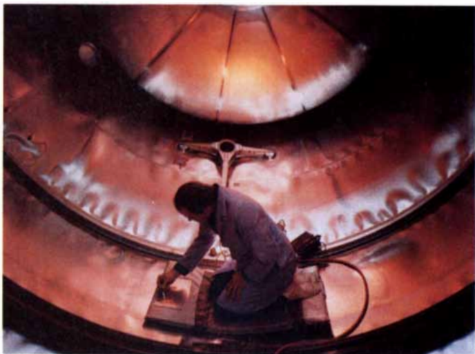
Inside the stainless steel skin of a Centaur upper stage, one of our craftsmen measures expansion and contraction stress. Unique technology makes the Atlas/Centaur the most efficient launch vehicle in use today.
