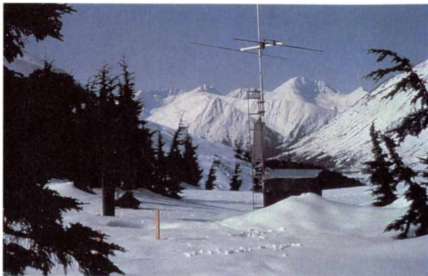
METEOR-BURST COMMUNICATIONS is used in remote areas of western states to transmit data on snow accumulations.
