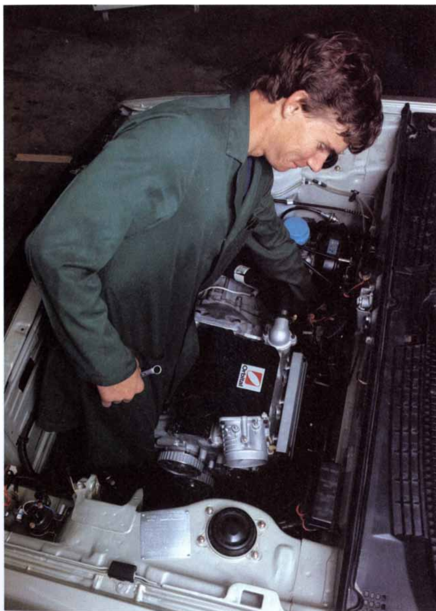
TWO-STROKE ENGINE developed by the Orbital Engine Company in Australia is so compact that it leaves enough room in an engine bay to accommodate a man. If the design can be made to meet emissions standards, it will help conserve fuel.
