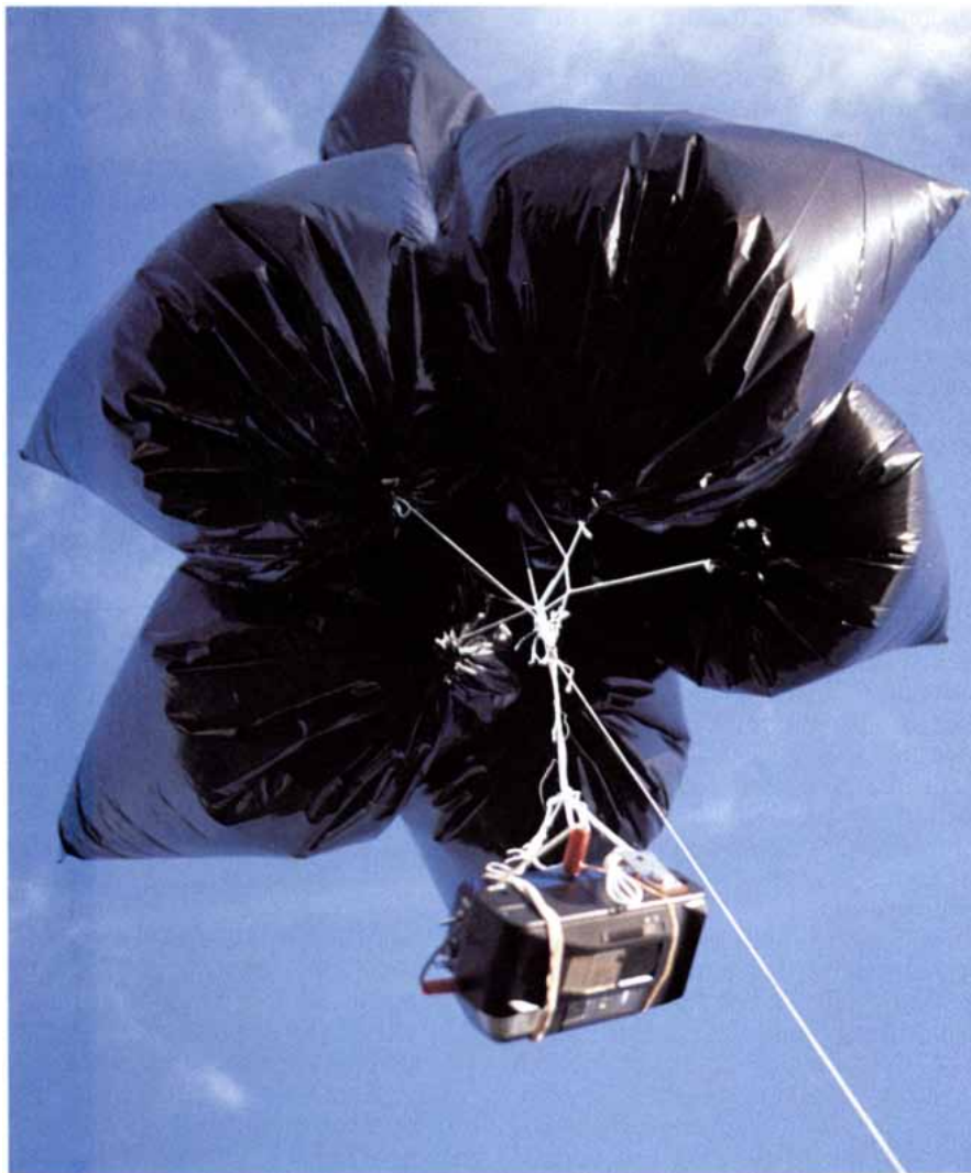
A camera payload suspended from a blimp (left) and a cluster of helium-inflated trash bags (right)
