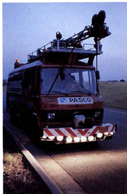
MACHINE VISION uses a boom-mounted camera to look for pavement damage.
