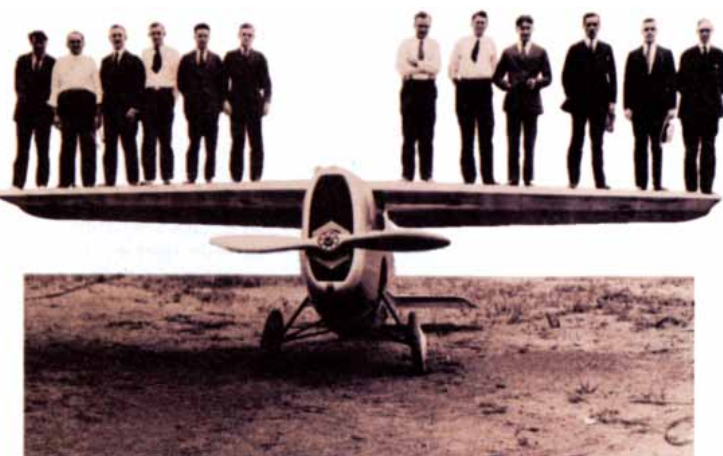
The RB Racer, made by Dayton-Wright Airplane Company, was the first aircraft to have fully retractable landing gear. Dayton-Wright became an early part of General Dynamics.
