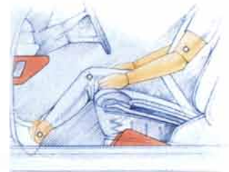
A wedge-shaped seat insert and padded knee bolster help reduce impact injuries.
