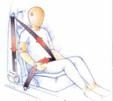
In certain impacts, front seat belts are tightened by emergency tensioning retractors.
