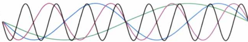
A Fourier transform breaks a signal into continuously repeating components at various scales, and so it is unsuitable for representing signals that change suddenly over time.
