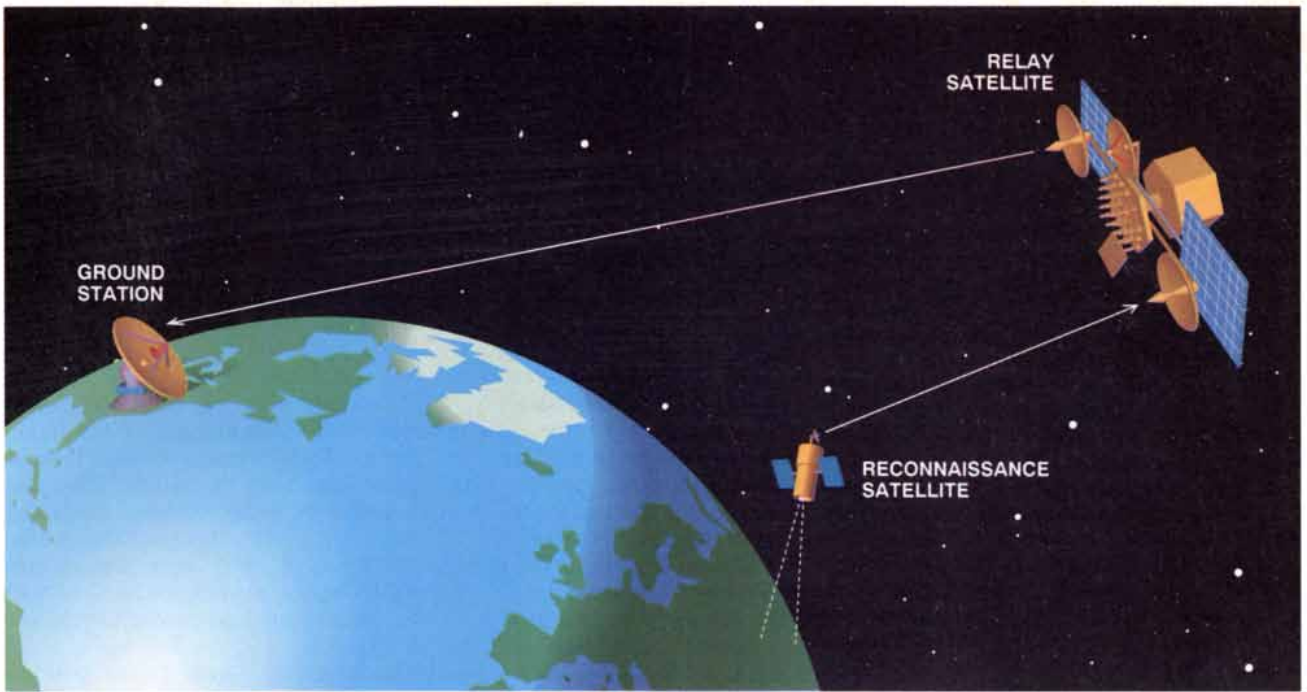
RELAY SATELLITES , such as the Tracking and Data Relay Satellite System, act as the intermediaries between satellites and ground stations. Relays speed the flow of data to the earth and complicate the interception of signals by enemies.
