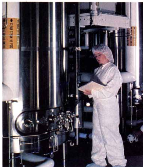
GROWTH FACTORS are made in mammalian cell-culture tanks at Genetics Institute, Inc.
