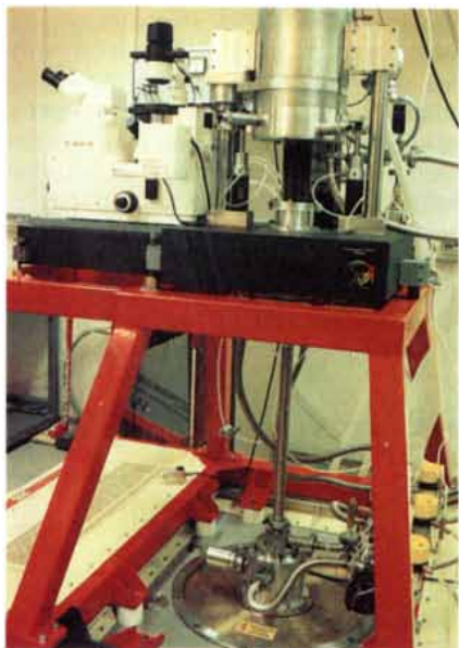
COMPACT IMAGING MICROSCOPE (left) developed at the universities of Göttingen and Aachen incorporates a plasma X-ray source; it has demonstrated a resolution of 1,000 to
