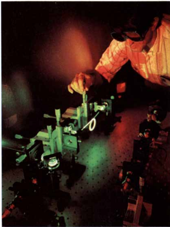
ERBIUM-DOPED OPTICAL AMPLIFIER (loop) is tested by Emmanuel Desurvire at AT&T Bell Labs.
