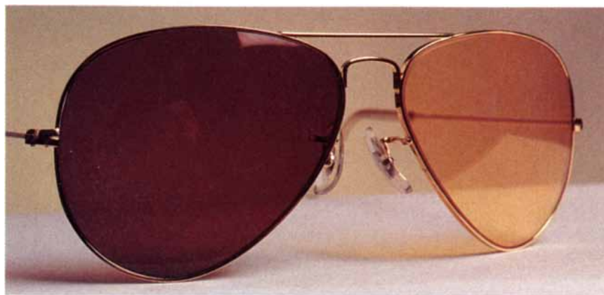
PHOTOCHROMIC GLASS finds primary use as lenses that darken outdoors. Here only one of the lenses has been exposed to ultraviolet light.
