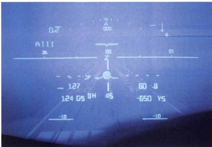
HEADS-UP DISPLAYS projected onto a glass screen in front of the pilot use navigational data from aircraft sensors and computers to make low-visibility landings, such as the one depicted in this flight simulator.
