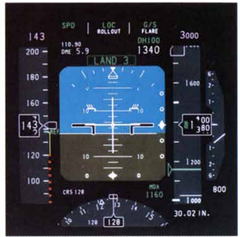
1980s GLASS COCKPIT in the Boeing 747-400 (left) has reduced by almost two thirds the instruments found in the earlier 747-200. The “blind flying” panel has been largely replaced by the primary flight display (right).
