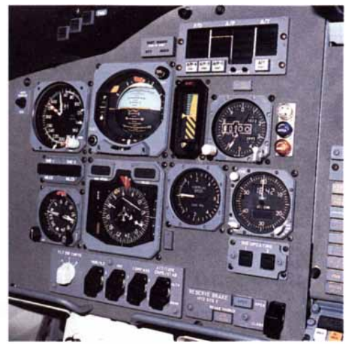
1970s ROUND-DIAL COCKPIT (left) on the Boeing 747-200 contains a panel with instruments (right) for altitude, airspeed, attitude, direction and rate of climb, among other gauges, that let a pilot “fly blind” in clouds or darkness.
