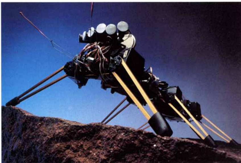
ROBOTIC INSECT named Genghis is a walking test bed of subsumption architecture. It can avoid obstacles and stalk people
