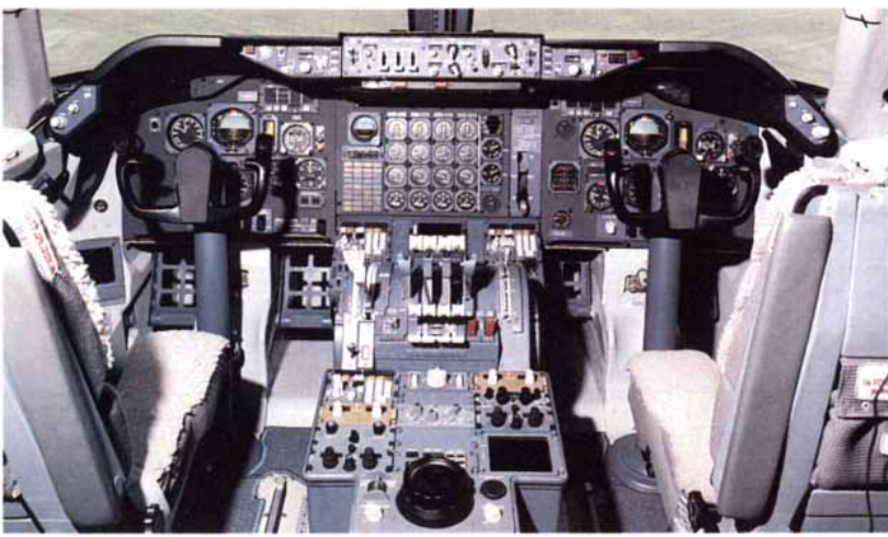
1970s ROUND-DIAL COCKPIT (left) on the Boeing 747-200 contains a panel with instruments (right) for altitude, airspeed, attitude, direction and rate of climb, among other gauges, that let a pilot “fly blind” in clouds or darkness.
