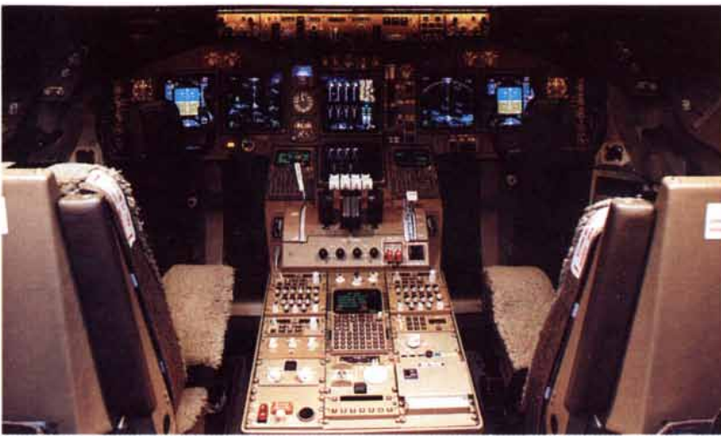
1980s GLASS COCKPIT in the Boeing 747-400 (left) has reduced by almost two thirds the instruments found in the earlier 747-200. The “blind flying” panel has been largely replaced by the primary flight display (right).
