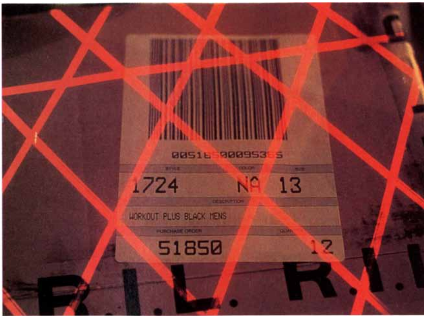
SCANNING OF BAR CODES is one component of the textile industry's Quick Response program. The scans provide information about the contents of a package to each member of the distribution chain, from supplier to retailer. The rapid transmission of data reduces inventory and enables the firms to adjust quickly to demand.
