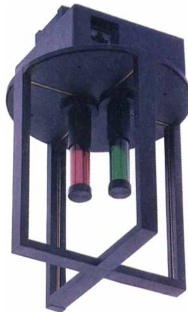
RADIO TRANSCEIVER links pads and other movable computer devices to the wired network. This unit, intended to be mounted on the ceiling, contains antennas in its crossed arms and two light-emitting diodes to signal its status.
