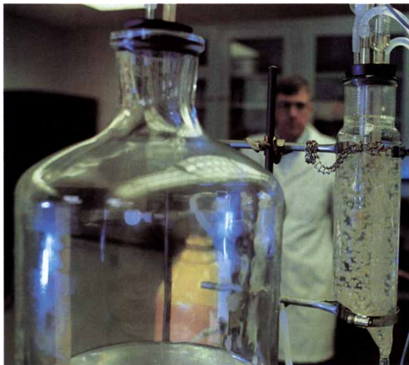
PLANT CELL BIOREACTOR , like the laboratory-scale model developed by Michael L. Shuler of Cornell University, may enable Pacific yew tree cells to yield the anticancer drug taxol. Photo: Jason Goltz.
