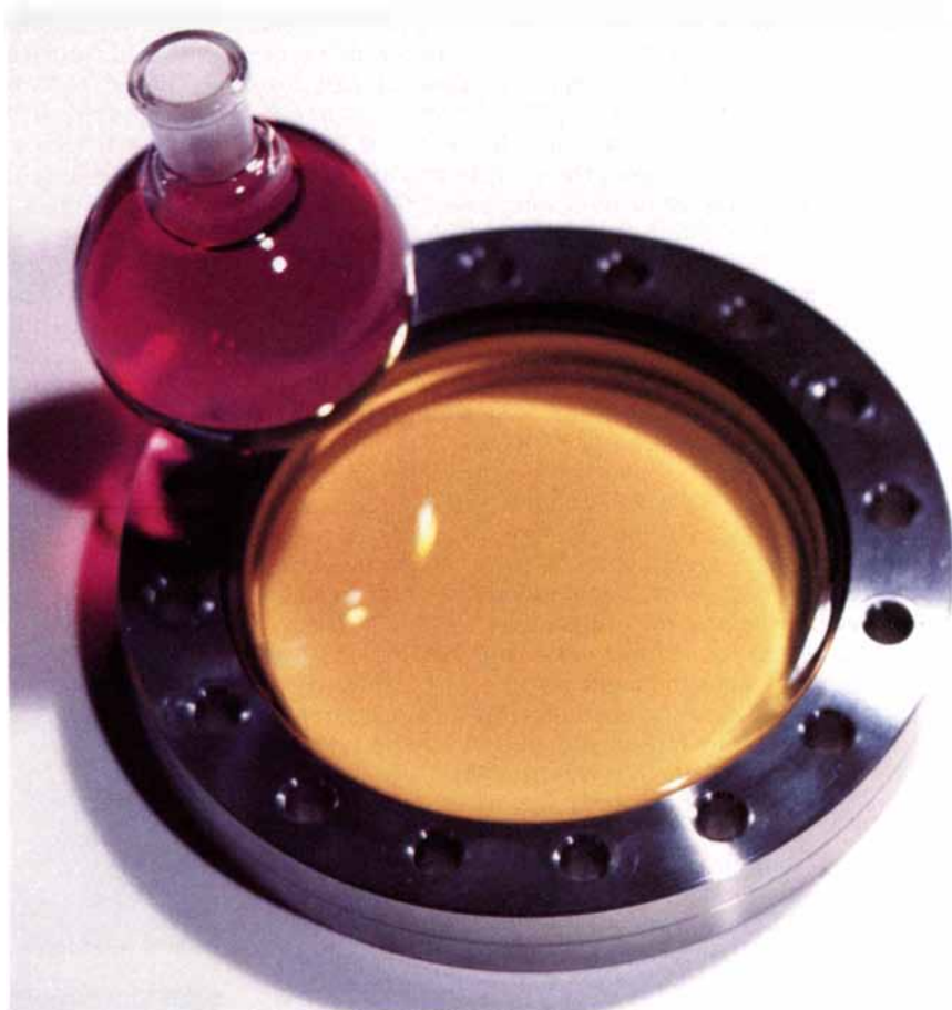
COLOR OF C_{60} depends on its form. This yellow film was sublimed onto a glass window that had been bolted to a vacuum oven. The benzene solution is magenta.
