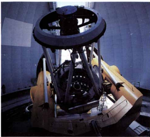
CANADA-FRANCE-HAWAII TELESCOPE on Mauna Kea (left) has been the test-bed for a prototype adaptive optics system. The telescope can now capture images of individual variable
