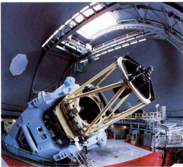
NEW TECHNOLOGY TELESCOPE in Chile ( left ) incorporates superb optics and a flexible primary mirror whose shape is adjustable; the instrument sits in an octagonal “dome” specially
