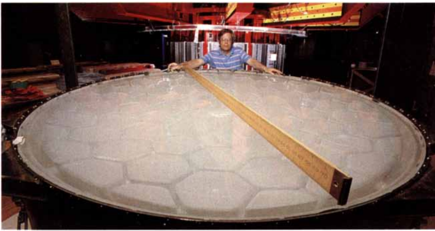
HONEYCOMB MIRRORS designed by Roger Angel of the Steward Observatory Mirror Laboratory offer one way of making reflectors that are large and rigid yet relatively lightweight. The mirrors are cast in a spinning oven that imparts a curved surface to the glass while it is molten, thereby simplifying the grinding process.
