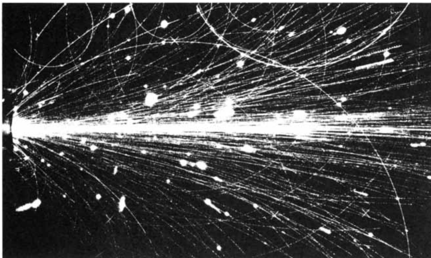
PARTICLE TRACKS produced in a collision between two nuclei yield information about the dynamics of the interaction. Such head-on collisions (left part of image) produce hundreds of charged particles, mostly protons and pions.
