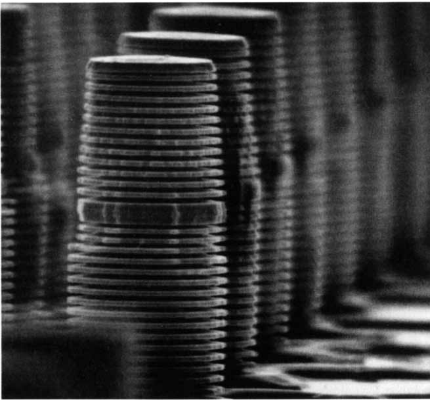
MULTILAYERED STRUCTURE of a microlaser is evident in a scanning electron micrograph. To show the structure, layers of aluminum arsenide have been etched preferentially, with the result that layers of gallium arsenide have larger diameters and project out. Such preferential etching is not done on a working microlaser.
