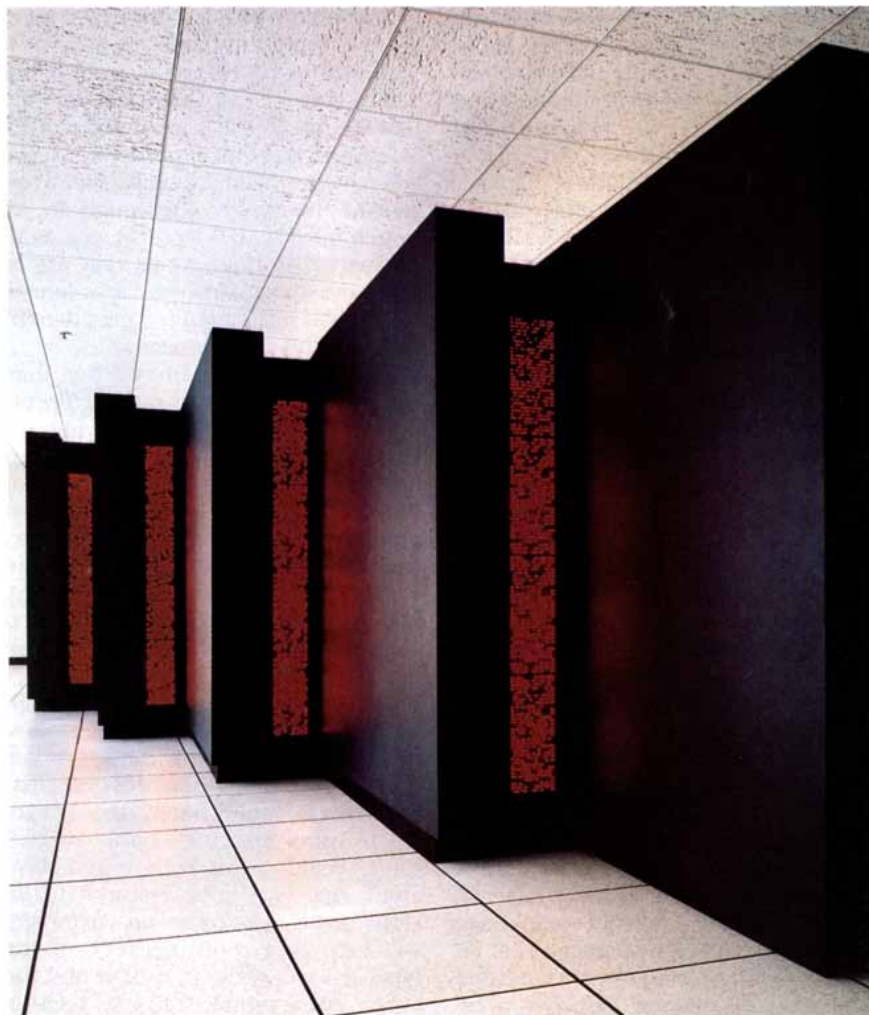
COMPUTERS should not look like refrigerators, Danny Hillis declares. This version of his new supercomputer uses 1,024 processor nodes. Photo: Steve Dunwell.
