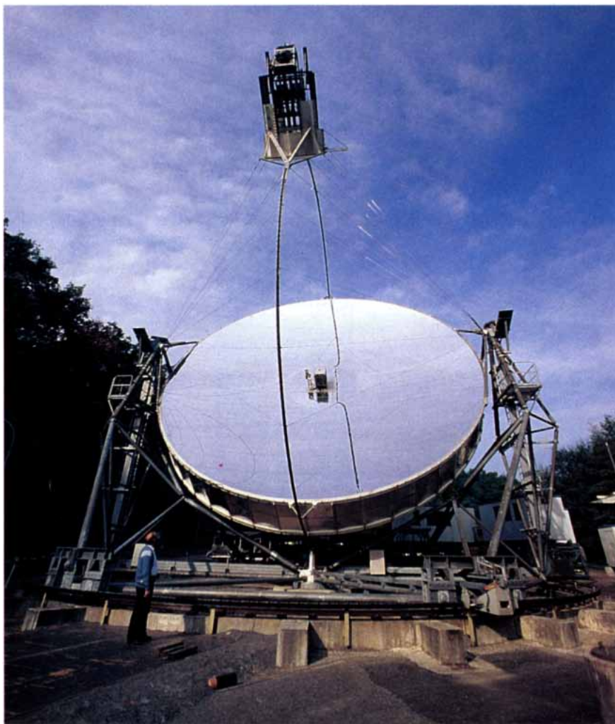
CONCENTRATED SUNLIGHT can be produced by a solar furnace ( top ) or a solar dish ( bottom ). The furnace intensifies terrestrial radiation up to 10,000-fold and is capable of delivering tens of thousands of watts of power. The dish yields up to 150,000 watts. This furnace is at the Weizmann Institute; the dish, located near Stuttgart, is operated by the German Aerospace Research Establishment.
