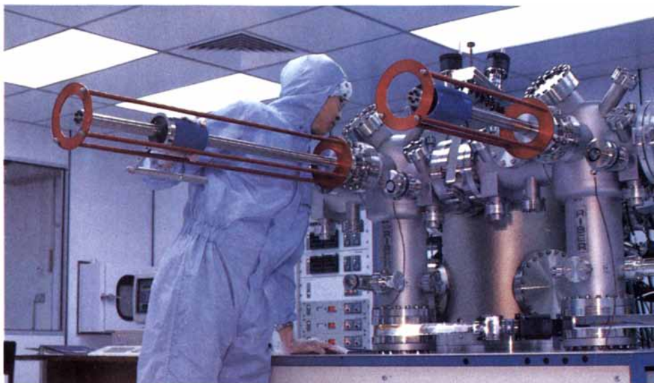
Preparation for growth of III-V compound semiconductor epitaxial layers
