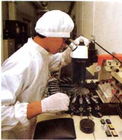
Highly-skilled personnel at the Probe Station characterizing device performance
