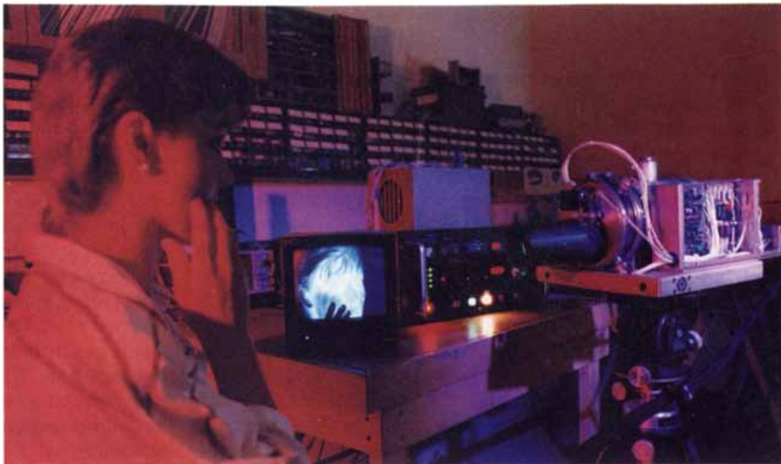
PLATINUM-SILICIDE INFRARED CAMERA is shown imaging the technician who wired the device. The thermal imprint left by touching the hand to the face is seen in the infrared image displayed on the monitor. Next to the monitor is the electronic control box used to focus and adjust the image. The silvered bulk of the camera is the dewar that cools the array of 39,040 detectors (not shown). Both the array and the readout circuitry fit on a single chip about the size of a dime.
