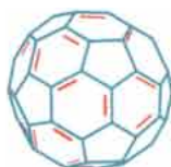
BUCKMINSTERFULLERENE (C 60 ) (0.0274) LARGE, STABLE, HOLLOW MOLECULE THAT IS THE THIRD FORM OF PURE CARBON; HAS VARIED PROPERTIES WHEN COMBINED WITH OTHER ELEMENTS
