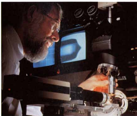
ASPHERIC TIP (projected on screen), at the end of a silicon fiber, was invented at AT&T by Herman M. Presby.
