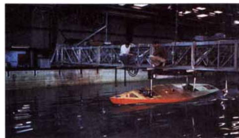
A 1/3.5 SCALE MODEL, 6 METERS LONG, BEING TESTED WHILE HEELED OVER WITH LEEWAY, IN THE ARCTEC TOW TANK, ESCONDIDO, CALIFORNIA.
