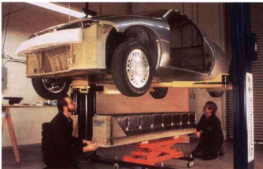
IMPACT , GM's new electric car, is powered by a state-of-the-art lead-acid battery, shown below the car at left. But Canada's Hydro-Quebec, teamed with 3M, is vying for a contract
