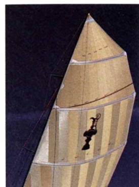
A KEVLAR MAINSAIL WITH RADIAL FABRIC PANELS THAT FOLLOW THE PRINCIPAL LINES OF STRESS. THE FABRIC WEIGHT IS HIGHEST AT THE TIPS, AND DECREASES TOWARD THE CENTER AND FROM THE OUTER EDGE (LEACH) TOWARD THE MAST.
