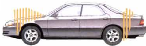
The front and rear crumple zones are designed to progressively give upon impact, rather than directly pass the energy on to the driver and passengers.
