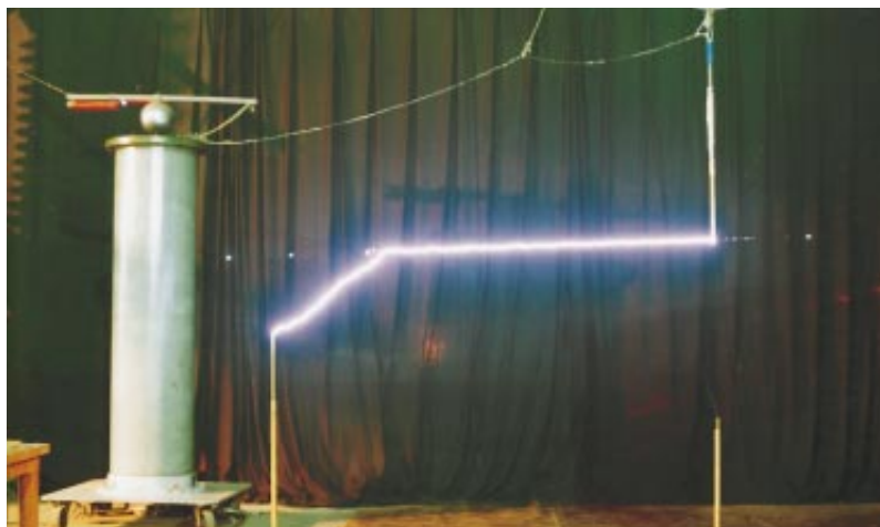
ARTIFICIAL LIGHTNING is guided by a laser to a grounded post at Japan Electric Power Industry's Central Research Institute near Tokyo.
