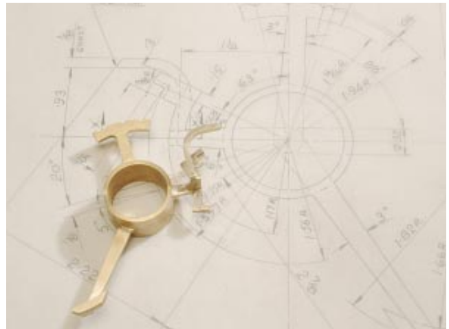
to verify the design of the engine's basic adding element. They also built 210 intricate bronze levers (right, shown atop a design drawing) for the carriage mechanism.
