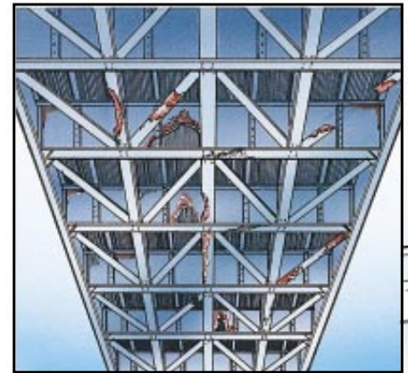
Bridge superstructure is susceptible to corrosion, water damage, metal fatigue and stress caused by vibration.
