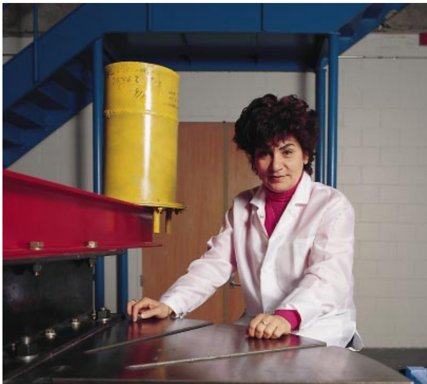
LIYA L. REGEL sits behind Clarkson University's new centrifuge, originally a boring mill designed to machine circular parts. The furnace used to grow crystals is mounted on the end of the centrifuge arm—a red, 10-foot-long I beam.
