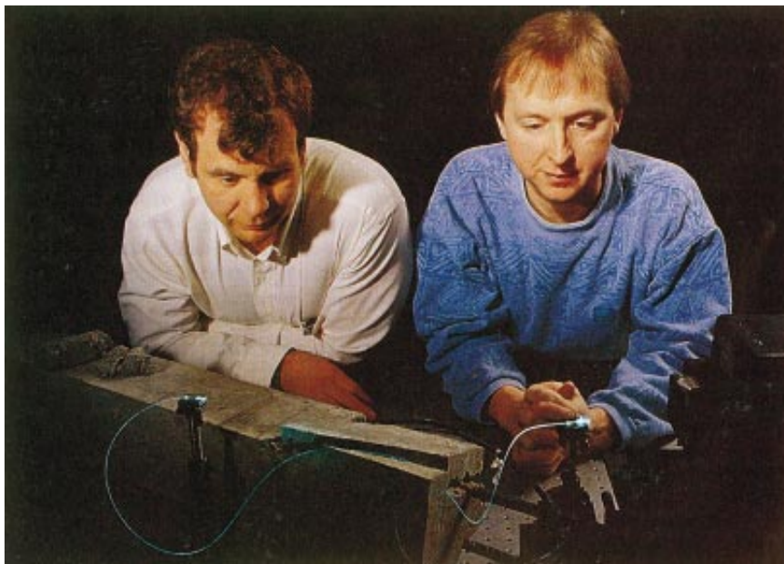
STRUCTURAL NERVOUS SYSTEM has been fashioned from a network of optical fibers by University of Vermont professors Dryver R. Huston (left) and Peter L. Fuhr. The fibers can detect the presence of cracks and flaws in concrete.
