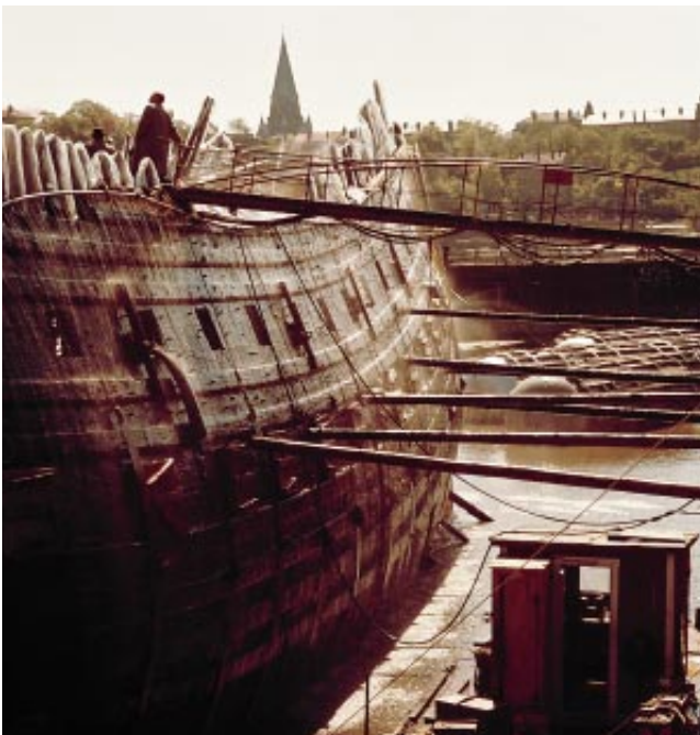
RAISED AT LAST , the Vasa 's hull was still held together by the original wooden pegs, although all the iron bolts and nails had rusted away many years before.
