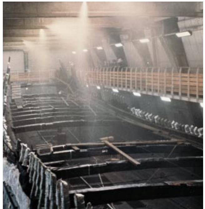
SHOWER OF POLYETHYLENE GLYCOL impregnated the Vasa over a period of 18 years. Smaller objects were treated more quickly by immersion in baths.
