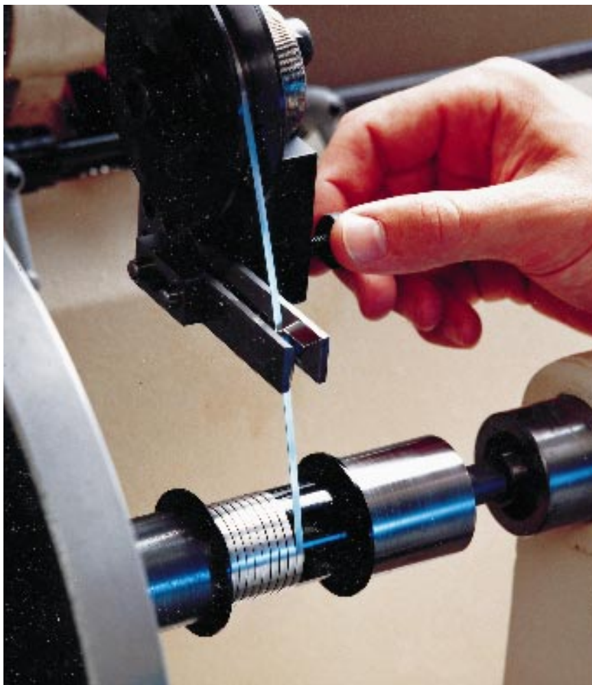
FLEXIBILITY of high-temperature superconducting wire is now sufficiently high that the wire can be wound into coils to make magnets.
