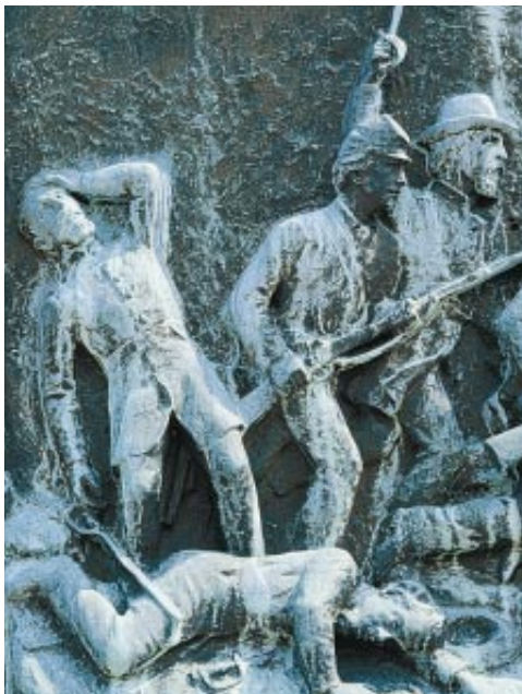
BRONZE MEMORIAL in Gettysburg National Military Park shows discoloring by acid rain.
