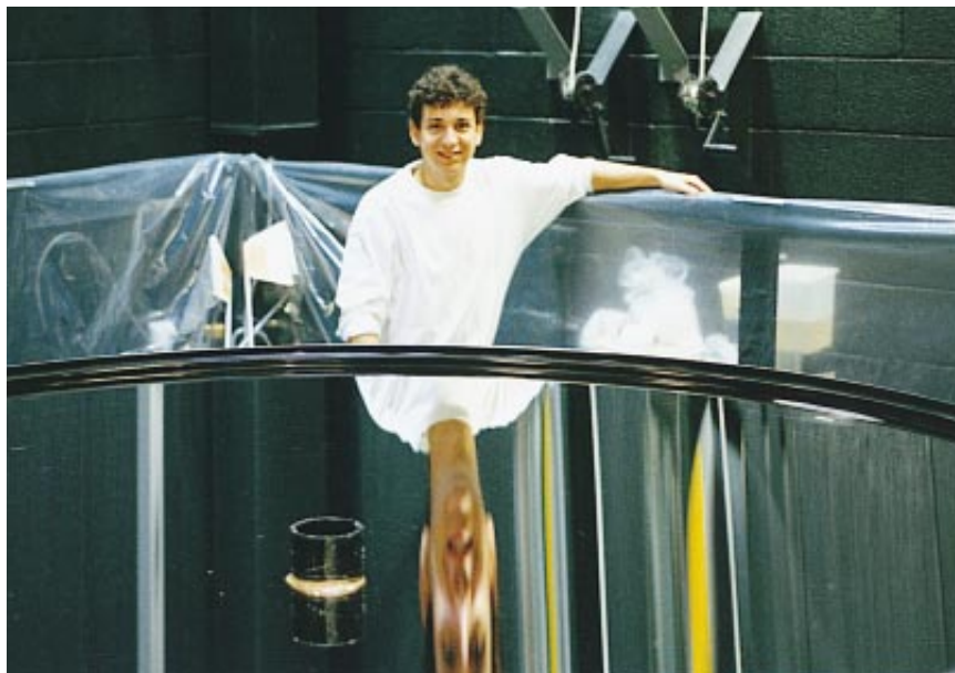
LIQUID MIRROR , tended by graduate student Luc Girard, acts as the receiver for an atmospheric monitor. The 2.7-meter mirror is at the University of Western Ontario.
