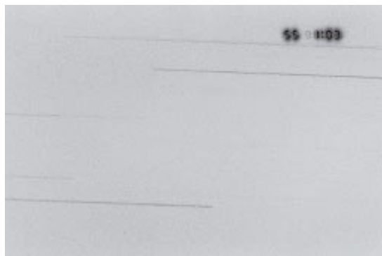
TEST RESULTS have shown that liquid mirrors provide superb optical surfaces. The interferogram ( top ) was obtained from a liquid mirror 2.5 meters in diameter. Computer analysis of this recording gives a false-color rendering that shows the surface contour of the 2.5-meter liquid mirror ( middle ). The stellar trails ( bottom ) were observed in 1987 using a 1.2-meter liquid mirror and a photographic camera.
