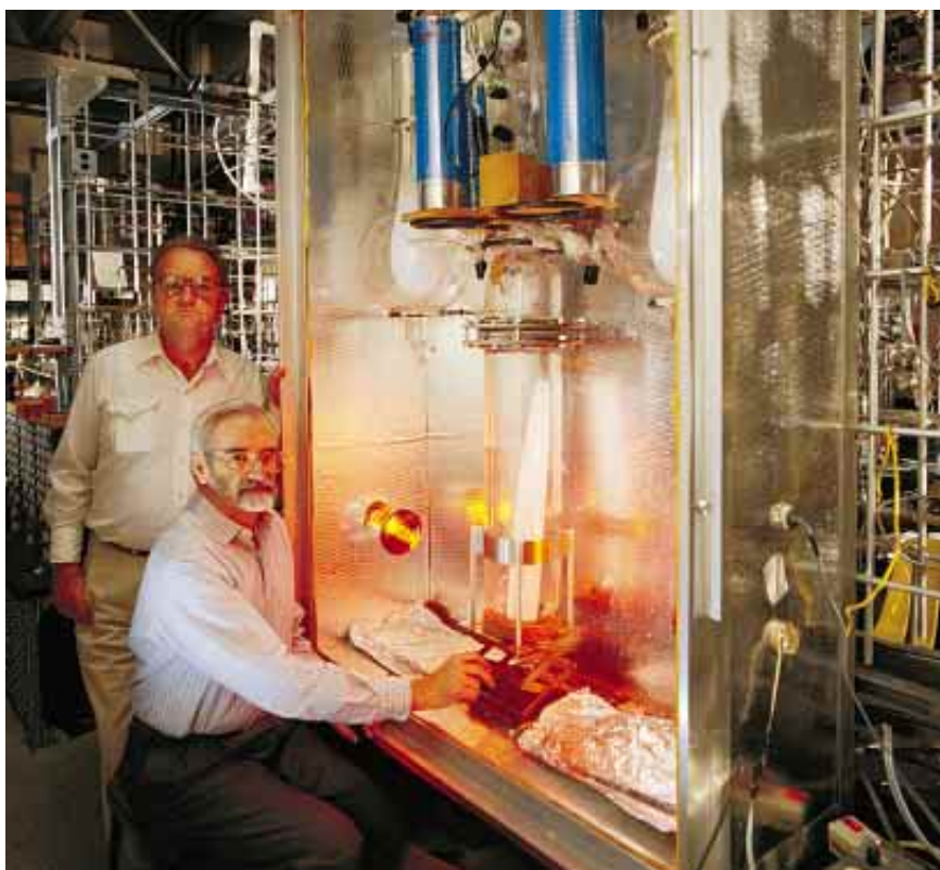
INNOVATIVE APPARATUS for measuring carbon dioxide in ice cores was developed by Alex T. Wilson (standing) and Austin Long of the University of Arizona.
