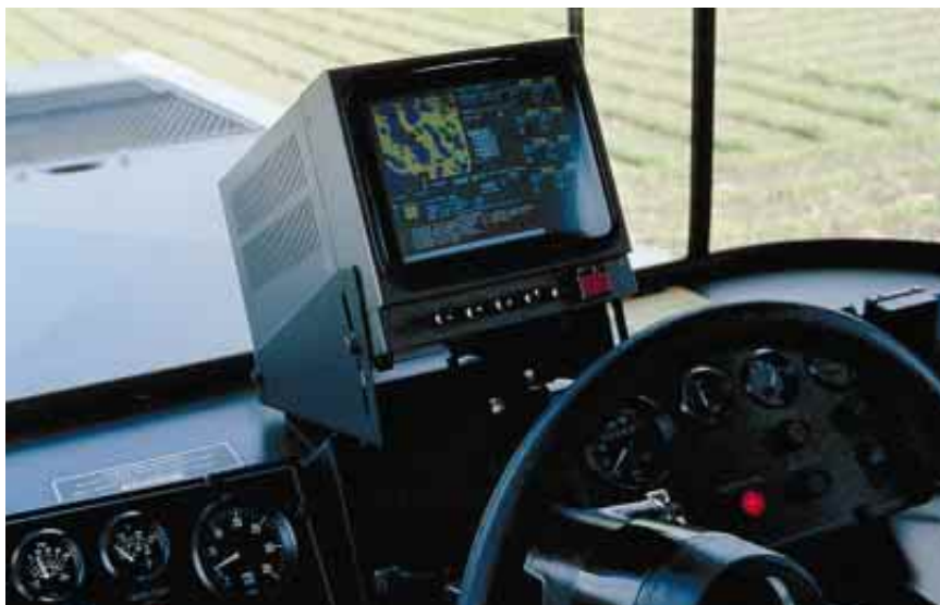
DASHBOARD COMPUTER on a tractor, carrying maps compiled via satellite, can now guide farmers in performing soil analysis and applying site-specific amounts and blends of fertilizer. Such technology saves money and increases efficiency.
