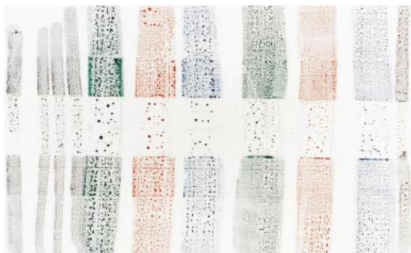
STICK TEST demonstrates how the ink from a felt-tip marker forms into tiny beads on Dow Chemical's fluorinated polymer (horizontal band), but the marker dye remains on the Teflon substrate on both the top and bottom.
