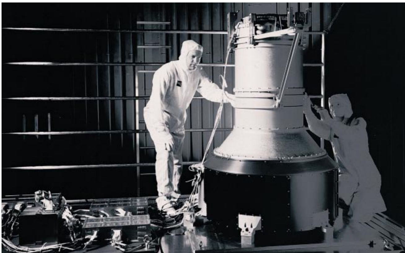
DEEP-SURVEY TELESCOPE and spectrometers are being prepared for integration with the EUVE satellite. The telescope takes long exposures of the sky in the direction of the earth's
