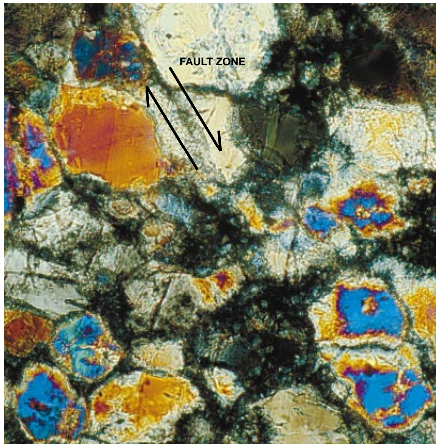
FAULT ZONE , produced by deforming a sample of mantle olivine, extends from the top left corner to the bottom right corner of the micrograph. An offset olivine crystal (white) appears on this fault in the top half of the image. The anticracks (yellow lenses in blue crystal) that generate the fault zone form perpendicular to the direction from which the sample is compressed. They grow throughout the material parallel to this direction.
