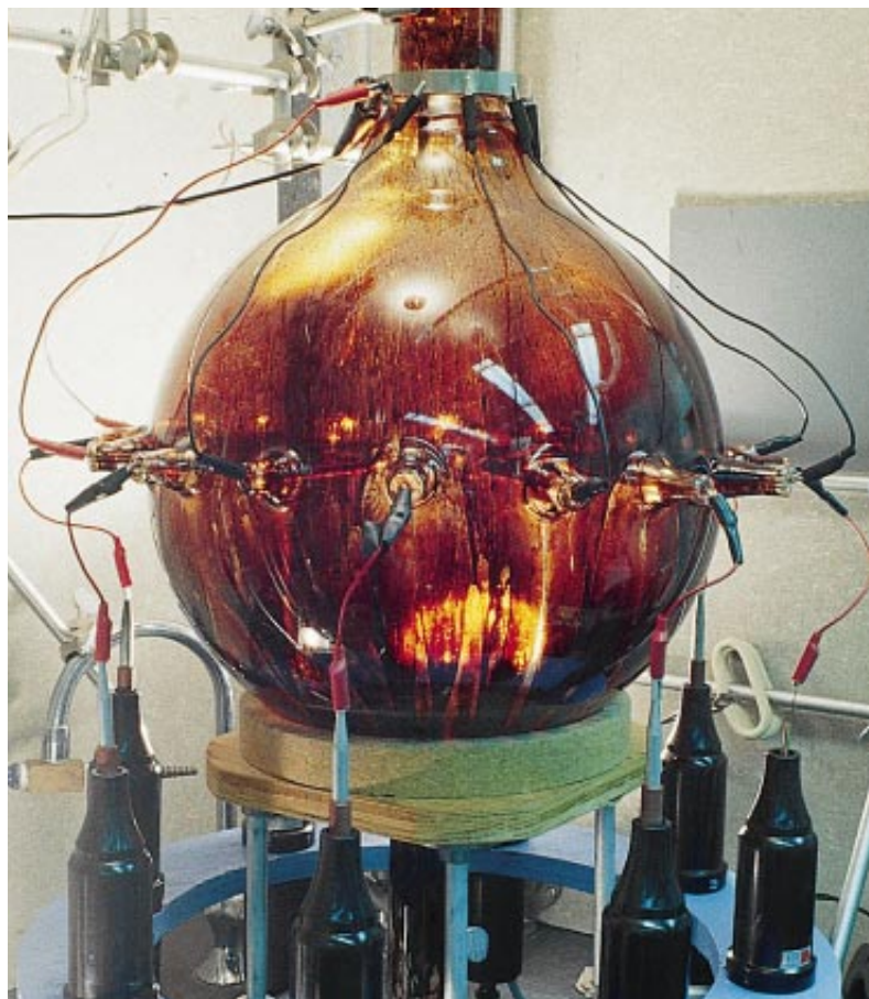
LABORATORY SIMULATION of Titan's nitrogen-methane atmosphere (left) yields a tarlike accumulation of complex organic molecules, which the author calls Titan tholin. Analogous chemical reactions may give rise to the haze that obscures Titan's surface (top right). The optical characteristics
