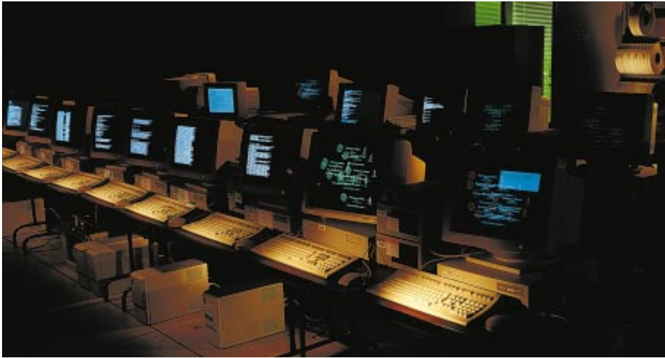
SERVER COMPUTERS for the Athena environment reside, for the most part, in this basement space at M.I.T.'s network operations center. A locked room (dubbed "the dungeon") within the server area holds the computer that runs the Kerberos key-distribution center.
