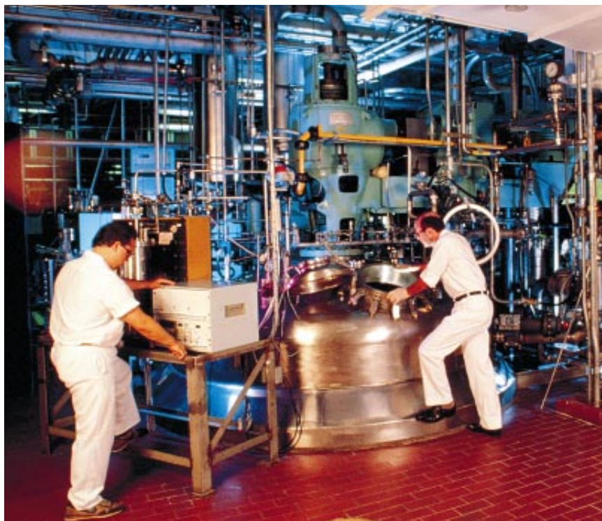
PRODUCTS of genetic engineering are manufactured on an industrial scale. Fermentation tanks at a Schering-Plough plant in New Jersey produce alpha-2b-interferon, approved in the U.S. to treat hepatitis C, Kaposi's sarcoma and hairy-cell leukemia.
