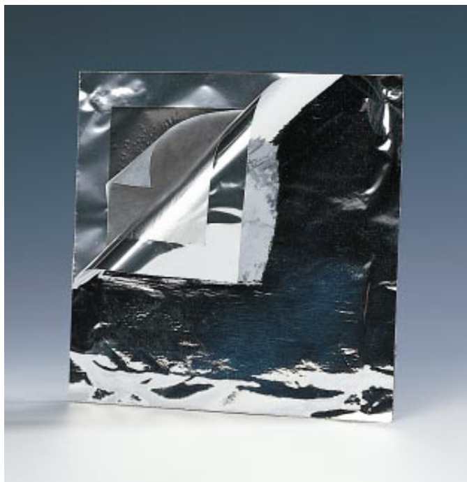
SOLID-STATE LITHIUM batteries may provide consumers with the ultimate cell: one that is light, cheap and energetic. This tiny model is approximately 150 microns thick.
