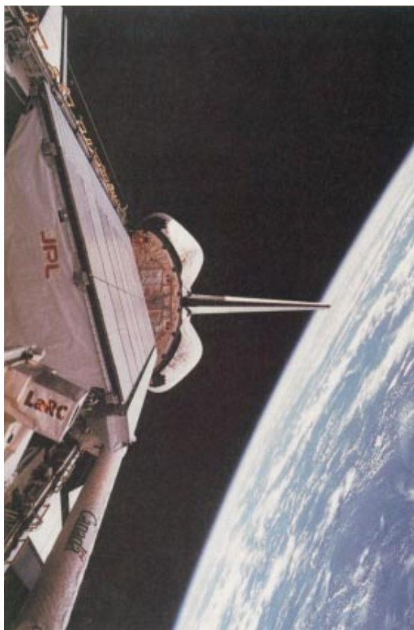
SPACE SHUTTLE ENDEAVOUR views the earth with radar. Visible on the shuttle are flat antenna panels that emit three wavelengths of radar, accompanying electronics (marked "JPL") and an apparatus for measuring atmospheric pollution from satellites (marked "LaRC").
