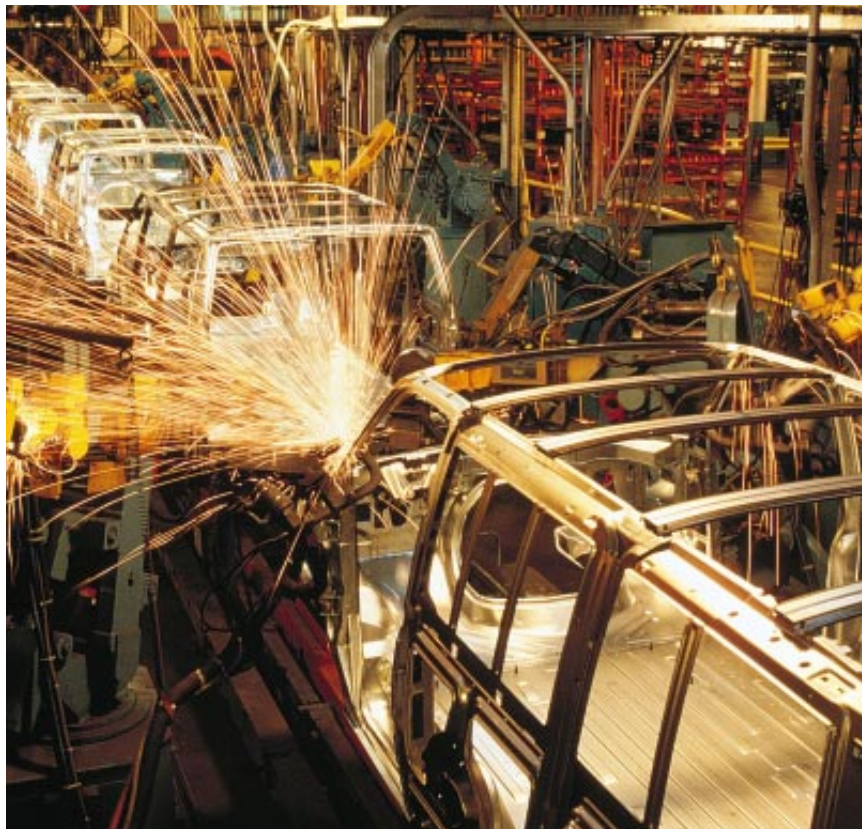
AUTOMATED WELDING SYSTEMS are crucial to the assembly of vehicle bodies. Innovations in the manufacturing process, such as use of laser welding that leaves joints smooth, will help raise energy efficiency of new models.
