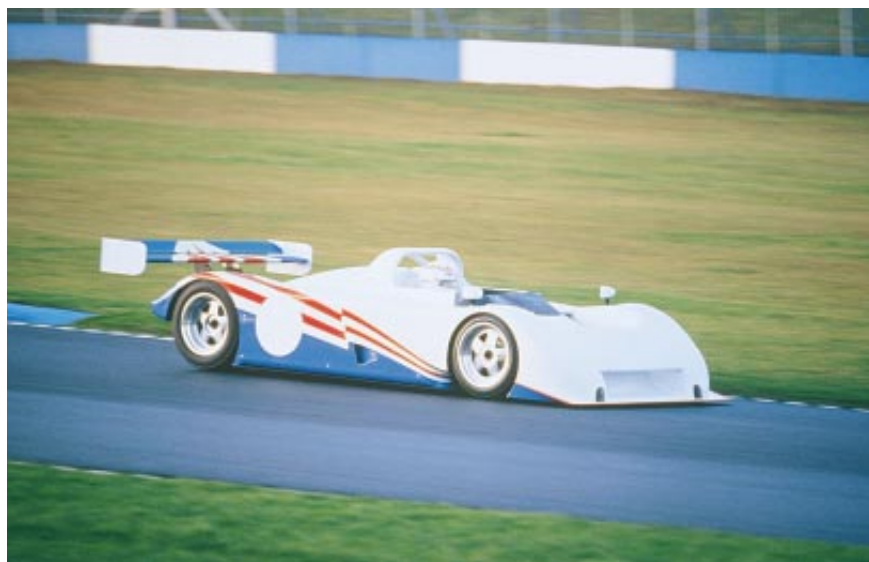
HYBRID RACING CAR recently designed by Chrysler Corporation uses a natural gas engine and an electromechanical battery, or flywheel. Passenger models using a hybrid approach are being studied by the Partnership for a New Generation of Vehicles.
